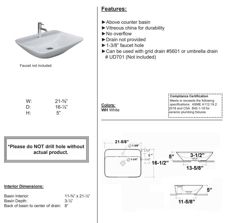
Dimensions of fixture are nominal and may vary within the range of tolerances established by AMSE Standard A112.19.2.2018 Dimensions and specifications subject to change without notice.
